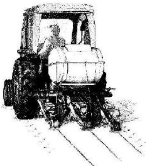
Slot seeding with adapted Stanhay/Gibbs drill
